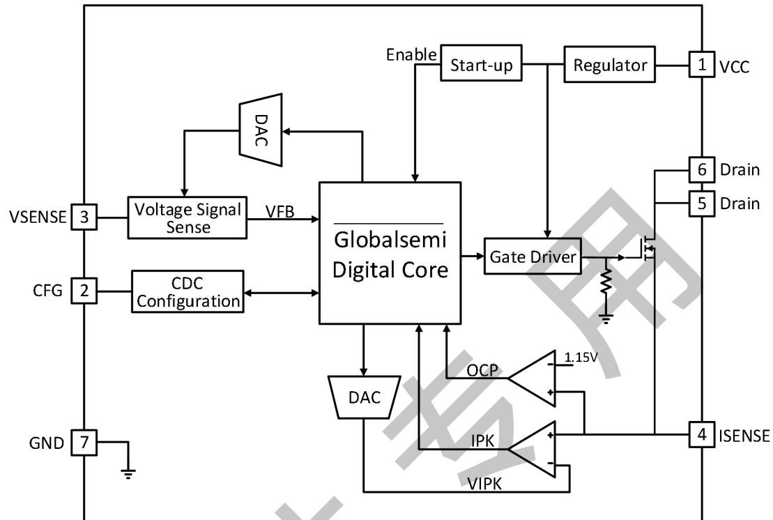
Figure3.1 G5237FT Functional Block Diagram
