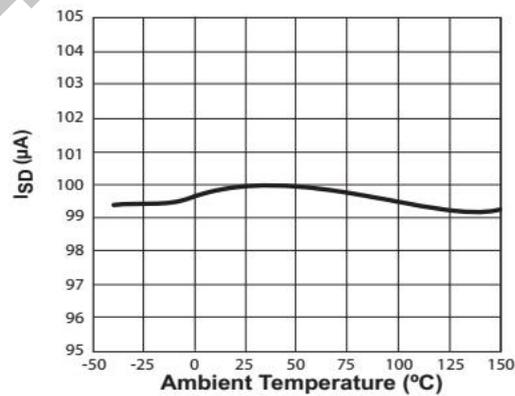
Figure 6.6 ISD vs. Temperature
