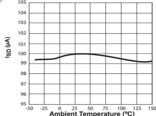
Figure 6.6 I<sub>SD</sub> vs. Temperature
