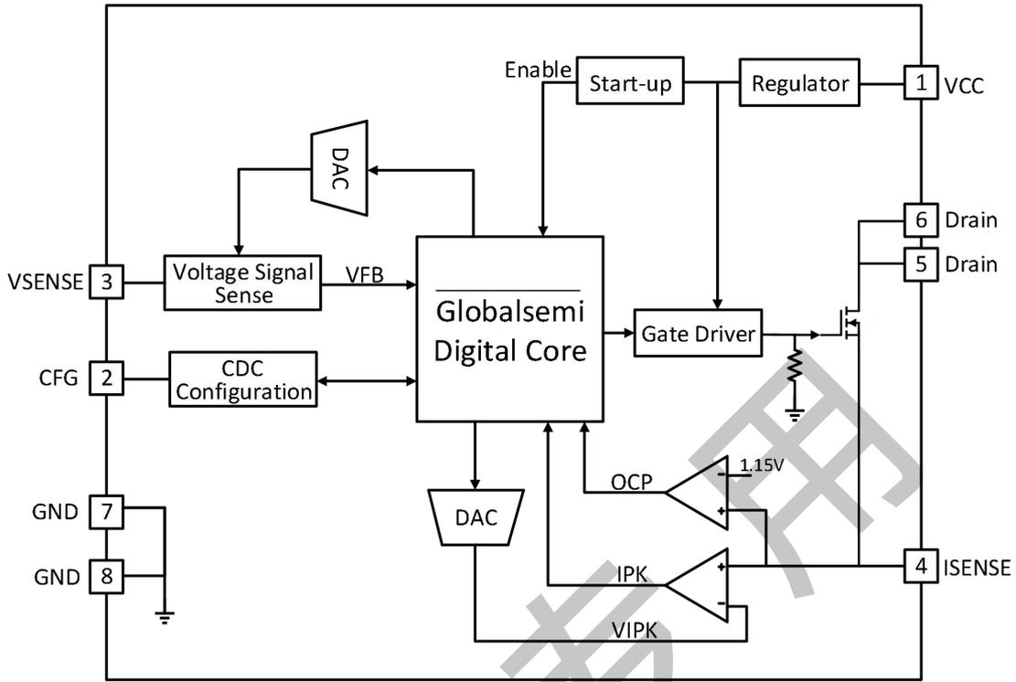
Figure3.1 G5137PT Functional Block Diagram
