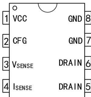
Figure2.1: G5137PT Series ( 8 Lead DIP8 Package)
