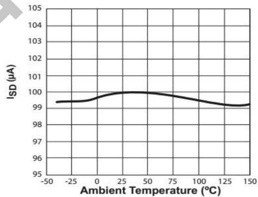
Figure 6.6 I<sub>SD</sub> vs. Temperature
